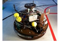
course) with both eyes, he is looking directly at it. If he goes off-path and only sees the object with one eye, he knows exactly which direction to turn back to. Kenny's eyes are also on a servo-driven turret that allows him to make precise angled turns with respect to an IR signal. For example, if he rotates his eyes 15 degrees to the right, when he rotates his body to find an IR signal, his body is 15 degrees to the left of where he would be if his eyes were looking straight.
